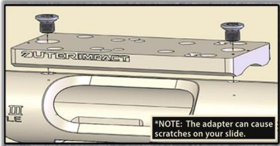
**Step 2:** Align M.R.A. with holes in the receiver. Fasten M.R.A. with Torx screws. Torque to **25 in/lbs.**
