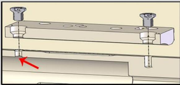
**Step 3:** Inspect the inside of the receiver to confirm the end of the torx screw does not interfere with the bolt.
