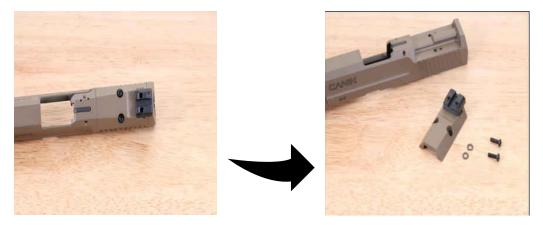
Step 3: Test fit the Red Dot sight to the OuterImpact adapter, utilizing the red dot pattern installation chart. Note: Make sure the screws do not stick out beyond the bottom of the adapter. After test fitting, remove Red Dot sight from the adapter.
