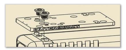
Note: Utilize blue liquid thread locker upon final installation of all threaded fasteners.
