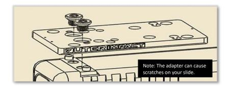
Note: The adapter has an intentional curve. This curve will flatten out when mounted.
