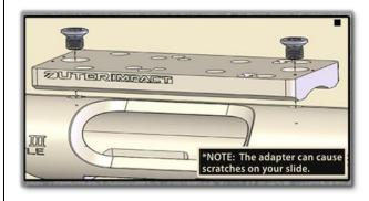
Step 2: Align M.R.A. with holes in the receiver. Fasten M.R.A. with Torx screws. Torque to **25 in/lbs.**
