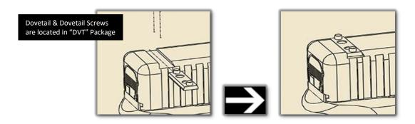
Step 3: Test fit the Red Dot sight to Outerimpact adapter. Note: Make sure screws do not stick out beyond bottom of adapter. After test fitting, remove Red Dot sight from adapter.
