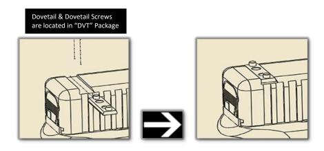
Step 3: Test fit the Red Dot sight to Outerimpact adapter. Note: Make sure screws do not stick out beyond bottom of adapter. After test fitting, remove Red Dot sight from adapter.
