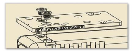
Note: The adapter has an intentional curve. This curve will flatten out when mounted. Utilize blue liquid thread locker upon final installation of all threaded fasteners.
