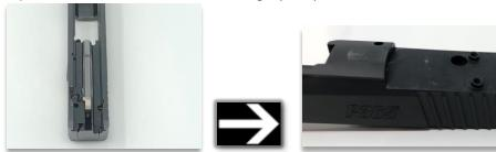
Step 2: Place Outerimpact plate onto the top of the slide.
