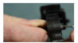
• Remove the parking brake mechanism from the OEM brake lever using the same method, the spring catch will need to be depressed twice to clear the lever. The parking brake will be installed on the new OuterImpact lever.
