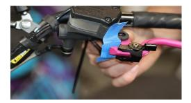
• Install the OuterImpact brake lever using either the OEM pin or the OuterImpact shoulder bolt. Be very careful of the brake switch. Remove tape after the lever is installed (if used).
