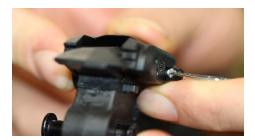
• Install the parking brake to the new OuterImpact lever using either the OEM pin or the OuterImpact shoulder bolt.
