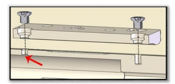
Step 3: Inspect the inside of the receiver to confirm the end of the torx screw doe not interfere with the bolt.
