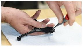
• Install the parking brake to the new OuterImpact lever. The spring for the parking brake rests on the backside of the new lever (seen below).
