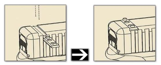
Step 3: Test fit the Red Dot sight to Outerimpact adapter, utilizing red dot pattern installation chart. Note: Make sure screws do not stick out beyond bottom of adapter. After test fitting, remove Red Dot sight from adapter.
