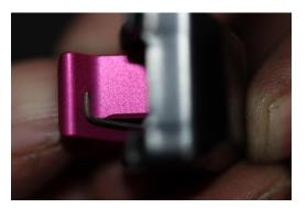
• Finish installing the OuterImpact brake lever on the assembly, reusing the retainer ring. Insert brake lever pin, being sure to slide the snap ring to sit in the groove on the pin.
