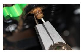
• Remove the brake lever pin and remove the lever.
