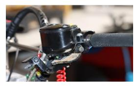
• Walk the retaining ring from the parking brake pin, taking care to not damage any of the ears as the retaining ring will be reused. Remove the parking brake.
