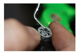
• When assembling parking brake, place the spring in the retaining hole and it will sit on the beak of the OuterImpact lever.
