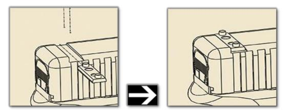
Step 3: Test fit the Red Dot sight to Outerimpact adapter, utilizing red dot pattern installation chart. Note: Make sure screws do not stick out beyond bottom of adapter. After test fitting, remove Red Dot sight from adapter.
