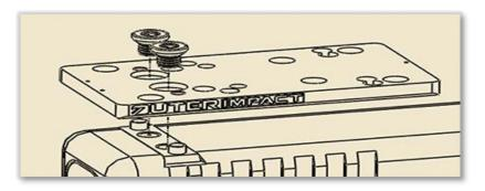
Note: Utilize blue liquid thread locker upon final installation of all threaded fasteners.
