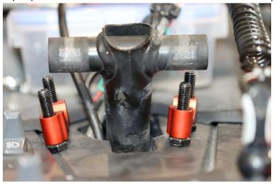
• You may need to tilt the riser forward to install the clamps and bolts, depending on clearance requirements. The clamps have an interior contour, the outside of the riser is flat.
