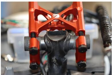
• When tightening the clamps, align the position of the riser to follow the same angle as the steering post. Then place the bottom bushing in place (if needed) before laying the handlebar in place. Place the top bushing in place and tighten the cap slightly.
