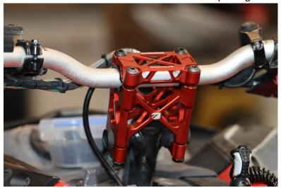
• Rotate handlebars to desired angle and align using the indicators on the cap prior to tightening completely.
